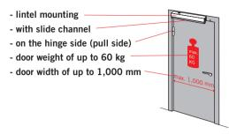
Most interior doors have a door width of less than 1,000 mm and a door weight of less than 60 kg.
