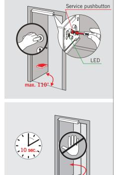
After 10 seconds, the door closes at low speed. An automatic learning cycle starts.
