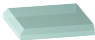
Flat edge with bevel oversized up to 45°
