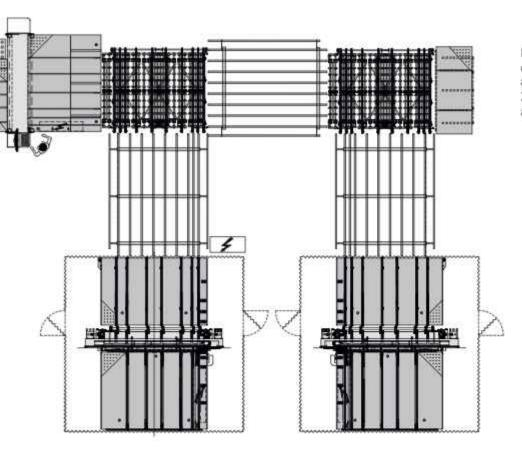
Loading, cutting and breakout line consisting of a loading system with automatic storage unit with gantry and X/Y laminated line with one leg in X and 2 parallel in Y. Manual unload.
