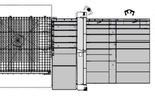
Loading, cutting and breakout line with fully automatic handling, except unload.
